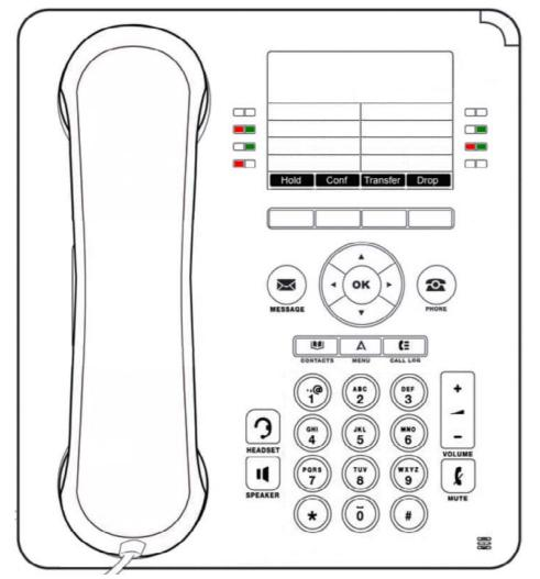
The phone supports 24 programmable call appearance/feature buttons. The labels for these are displayed in the main display and can be controlled by the adjacent buttons.
