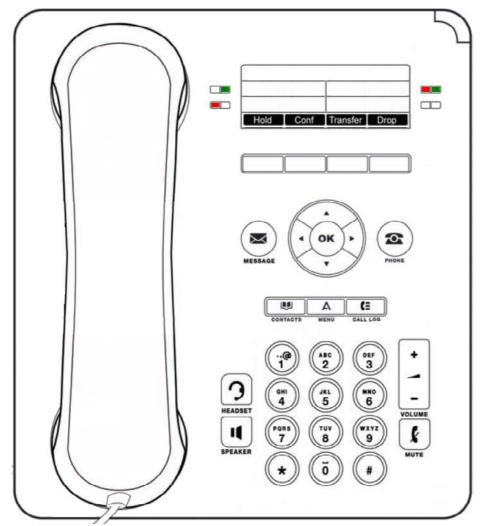
The phone supports 12 programmable call appearance/feature buttons. The labels for these are displayed in the main display and can be controlled by the adjacent buttons.
