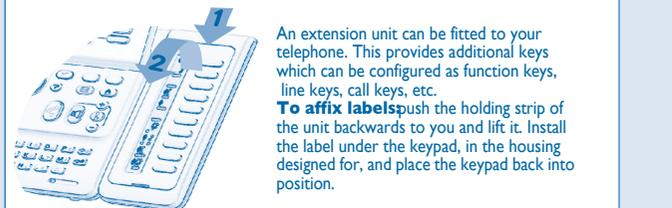
An extension unit can be fitted to your telephone. This provides additional keys which can be configured as function keys, line keys, call keys, etc.
